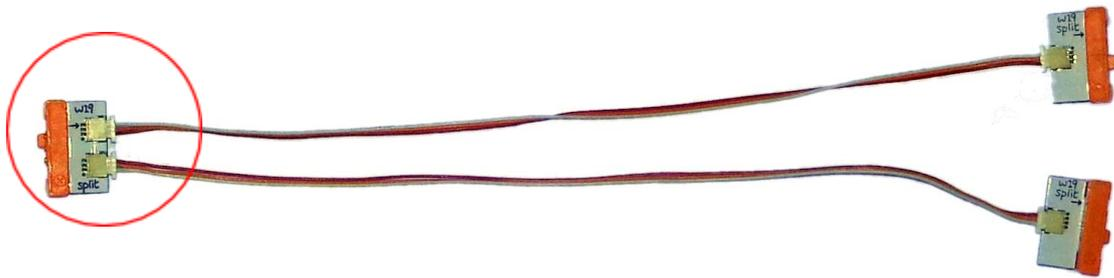
Unplug the end where both wires connect, circled in red on the left of **Figure 2**, by pulling on the white connector.
