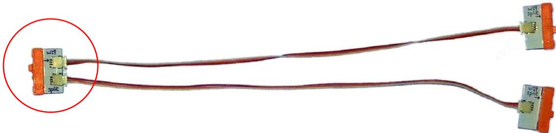
Unplug the end where both wires connect, circled in red on the left of **Figure 2**, by pulling on the white connector.
